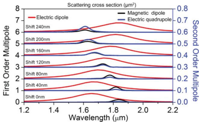
FIG. 4. (Color online) Scattering cross sections ( $\mu\text{m}^2$ ) of the electric dipole (left axis) as well as the electric quadrupole and magnetic dipole (right axis) of the shift-bar particle in water for different shifts.
