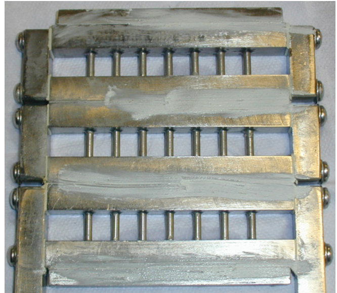
FIG. 6. (Color online) Negative acoustic index metamaterial sample. The RS resonator rods are visible, while the HH are formed in the horizontal stainless-steel bars leaving only the neck openings visible.
