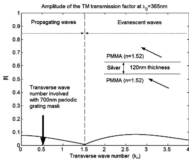
FIG. 1. Computed amplitude transfer function of 120 nm slab silver. It is clear that both propagating and evanescent waves are attenuated by silver slab, leaving no advantage of resolving subwavelength features.
