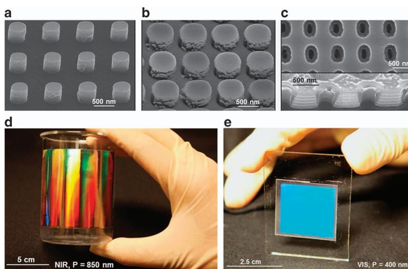
**Figure 1** (a–c) SEM images of nanoimprint lithography-formed fishnet structures (a) before and (b) after deposition of multilayers of Ag/MgF<sub>2</sub>, and (c) after removal of the polymer scaffold. (d, e) Macroscopic optical images of (d) telecom band and (e) visible band 3D NIM structures. Adapted with permission from Gao *et al.*<sup>4</sup> Copyright 2014 American Chemical Society.
