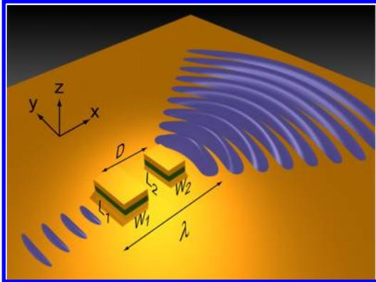
**Figure 1.** Schematic of the compact magnetic antenna that can generate directional SPPs. The antenna consists of two magnetic resonators with different geometries. Each magnetic resonator is made of a metallic nanodisk that is separated from a metal substrate by a dielectric layer.
