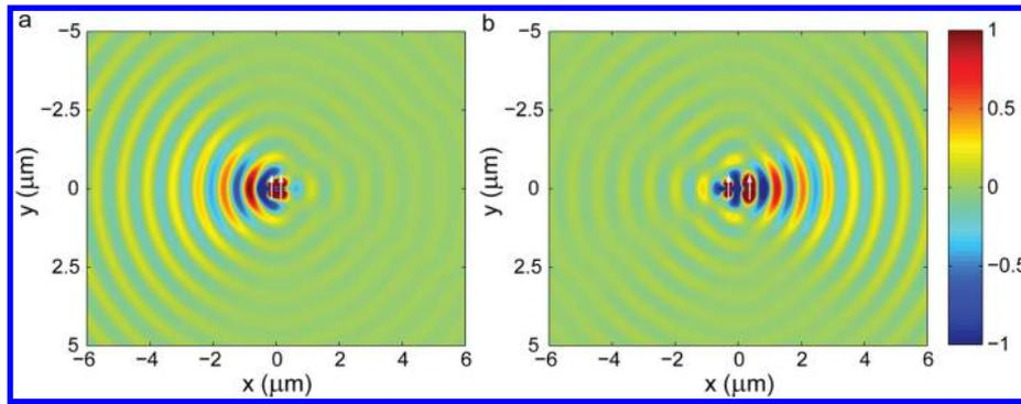
**Figure 3.** The electric field distribution of SPPs under the magnetic dipole approximation. The distance of the two dipoles is (a) 300 nm and (b) 600 nm, respectively. The phase difference of the two dipoles at a wavelength of 820 nm is taken from Figure 2c.
