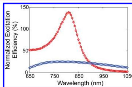
**Figure 5.** The spectral response of the normalized excitation efficiency of SPPs for a magnetic resonator (red circles) and a nano aperture (blue diamonds). The length and width of the magnetic resonator are 250 and 150 nm, respectively. The aperture is milled through a 50 nm gold film but with the same physical dimension.
