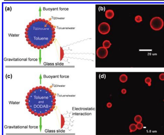
**Figure 1.** Scheme of microdroplet structures. Cross-sectional views of a QD-stabilized microdroplet and forces affecting its stability for (a) method 1 and (c) method 2. Corresponding confocal microscope images of QD-stabilized microdroplets (c) method 1 and (d) method 2. Although QDs might introduce some surface roughness of the microdroplets, a relatively homogeneous interface between two liquids can still be preserved even in the presence of QDs.
