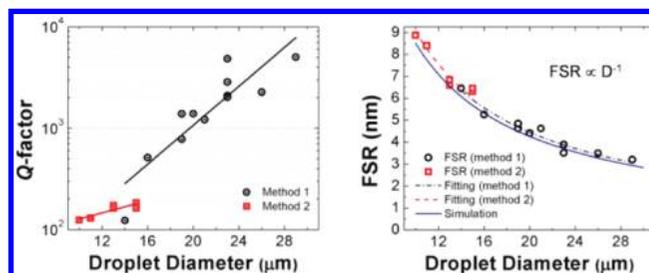
**Figure 3.** Size dependence of  $Q$ -factors and losses (method 1 and method 2). (a)  $Q$ -factors from PL spectra with various sizes of microdroplets. (b) Mode distance at maximum wavelength with various sizes of microdroplets.
