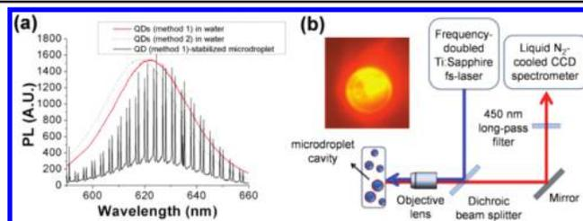
**Figure 2.** (a) PL spectra of ligand-exchanged QDs (method 1 and method 2) and a WGM (a 23- $\mu\text{m}$ -sized microdroplet with QDs modified by method 1), which were excited at 405 nm. (b) Bright field image of WGM microdroplets together with a scheme of the photoluminescence measurement setup.
