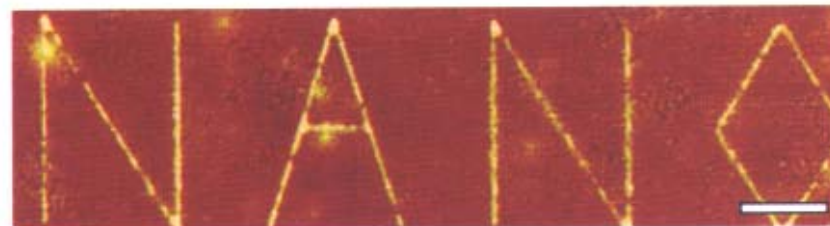
An AFM image of features etched onto a photoresist by evanescent waves focused by a silver superlens. Scale bar = 2 \mu m. (Adapted with permission. Copyright 2005 American Association for the Advancement of Science.)
